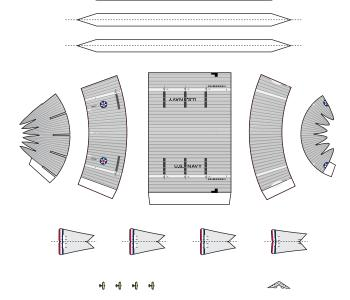
Fold the four fins and glue in place. The bottom fin is slightly different from the others, with tiny windows of an observation post used when landing the Akron.
